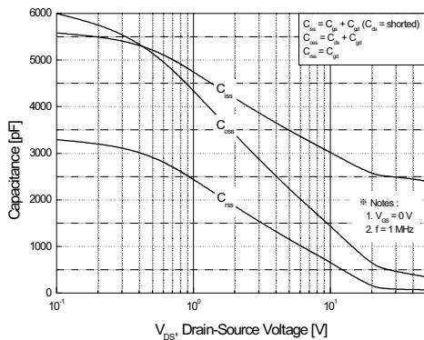
**Figure 5. Capacitance Characteristics**
