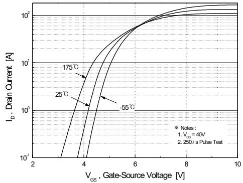
**Figure 2. Transfer Characteristics**
